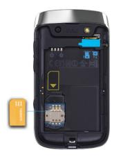
Slide the SIM card into the slot.
